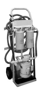
element. Fluid transfer using this cart may be done while the system is running.
